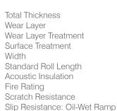
2.00mm 0.70mm HyperGuard+™ Sanitec ™ 2m & 4m 25 l/m Lw 7 dB 7.5kW/m<sup>2</sup> CRF Class T R10
